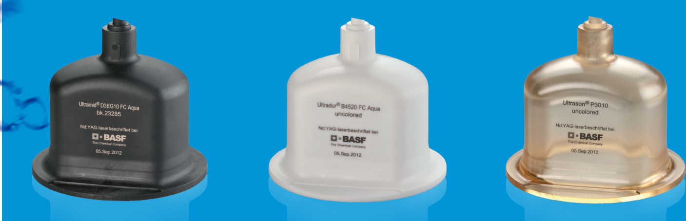
Fig. 3: Ultrasonic® Fatigue Testers made from Ultramid® D3EG10 FC Aqua (left), Ultradur® B4520 FC Aqua (middle), Ultrason® P3010 (right)
