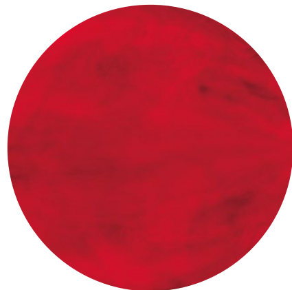
Fig. 5: Circular disk made of Ultraform® N2320 003 AT and 3.5% of batch C1 using a standard screw
