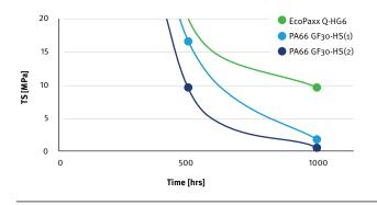
Figure 1— Tensile strength at weld line after 135°C aging in a 50% mixture of water/G13
