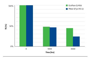
Figure 2 - Tensile strength after 120°C aging in a 50% mixture of water/G13
