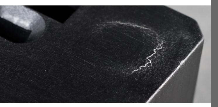
When such defects occur, it is important to verify that both the **Melt Temperature** and the **Back Pressure** are in accordance with the documented standard.
