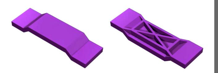
Gating into thick sections of the part will often improve the molder's ability to properly pack out the part. Increasing the size and number the gates used may also improve overall dimensional stability.
