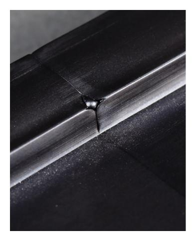
Cooler materials also have lower polymer chain mobility which significantly reduces the molecular chain entanglement where the two flow fronts meet.
