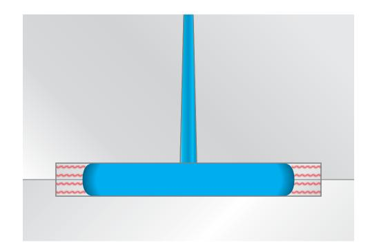
Static vents can be machined on the sides of stationary components such as inserts and core pins. Dynamic vents can be added to moving mold components such as lifters, slides, and ejector pins. Porous steels, which allow air to pass through the cavity surface, can be inserted into cavity areas where burning is very likely to occur.
