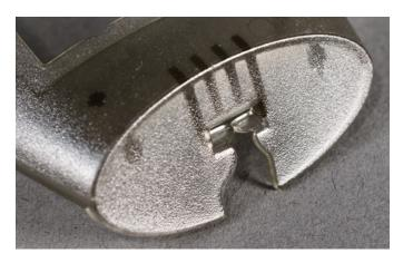
If 2nd Stage parameters are suspect, return the Packing Pressure to the documented standard.
