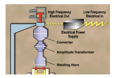
One of the two parts to be joined is placed into a stationary fixture. The top part is placed either on top of the lower part, or is placed into the **Welding Horn** above.
