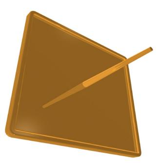
Due to their size, sprue gates leave a large amount of vestige and are difficult to separate from the part. Separating the gate from the part often requires large gate cutters. To remove the vestige, parts often require a secondary operation, such as machining or filing.
