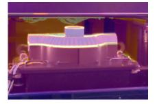
As part of the quality control process, Nexeo Plastics recommended adding thermal imaging to inspect the weld along the entire seam of the vent and ensure a water-tight fit.
