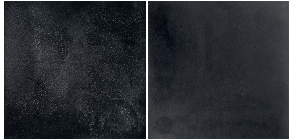
Fig. 7: Wet/dry alternating storage test showing resistance against humidity left: standard PPA/FR with visible surface defects due to migration of flame retardant right: smooth surface due to lowest migration of flame retardant with Ultramid® Advanced N 30% GF FR
