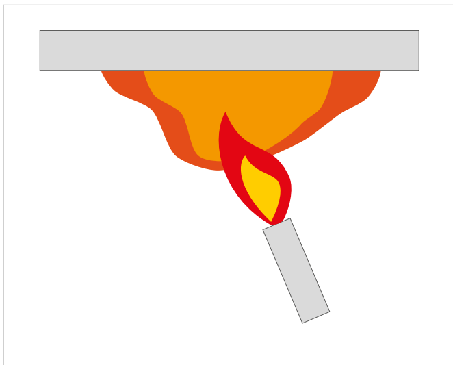
Fig. 7: UL 94 5V (or DIN IEC 60695-11-20 ), application of a 125 mm (500W) test flame to plaques 150 · 150 mm 2
