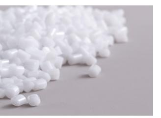
CYREX<sup>®</sup>, an opaque acrylic-polycarbonate alloy, is a unique marriage between acrylic and polycarbonate where the final product exceeds the sum of the two components that make up the product. The most notable property advantage of CYREX<sup>®</sup> alloy over either of its components is in notched izod impact strength. It is an ideal material for applications which require excellent toughness CYREX<sup>®</sup> alloy offers:
