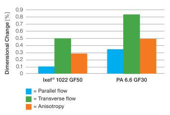
Test sample: 40 × 20 × 2 mm Test conditions: 750 bar, 280 °C/536 °F Tooling: 120 °C/248 °F, direct gating
