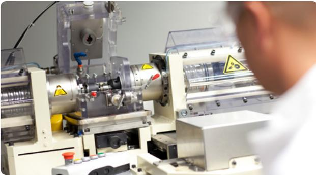
In order to effectively carry out this advanced testing, DSM modifies its testing equipment to include precise temperature control in addition to pressure and sliding speed variables to best approximate practical applications.
