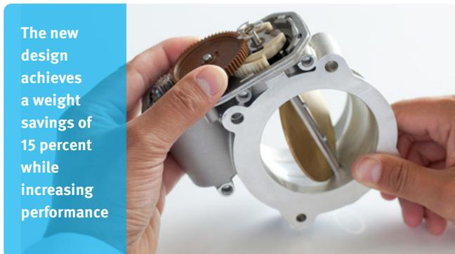
The new design achieves a weight savings of 15 percent while increasing performance, allows for a hood line of up to 5 millimeters lower to save fuel due to less resistance, and delivers a two-year gain in service lifetime to five. The new electronic throttle body, which entered the market in 2010 model year vehicles, meets all interface and performance requirements for all engine management systems, and will replace all existing gasoline and diesel actuators in GM vehicles by 2015.
